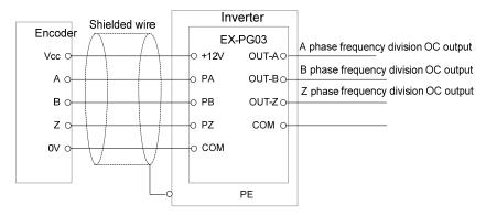
For the differential motor speed feedback encoder whose power supply is +5V, please adopt the V&T PG feedback card EX-PG02.If the inverter needs to transmit the motor rotation speed to other equipment for calculation or speed measurement in addition to vector control 2 with encoder speed feedback, please adopt the V&T feedback card EX-PG04 with frequency division output.
