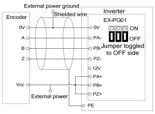
Connection diagram of EX-PG03 card (Does not support external power supply)
