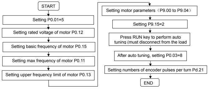
After setting and test by the above steps, should JOG running first. If working order , the user can set other function according to V6-H user manual, for details, refer to user manual of V6-H high performance vector control/torque control inverter.
