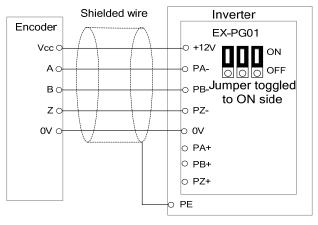
Connection diagram for EX-PG01 card adopting external power supply
