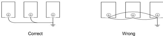
Figure 2-2 Grounding wiring
