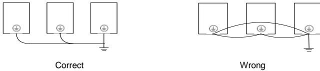
Figure 2-2 Grounding wiring
